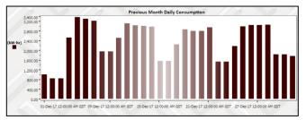
For ex, if the consumption in a weekend is almost equal to a weekday or if the after-work hours pattern is equal to the unoccupied hours, we can study through the history log to find the root cause of the deviation. Every month, L2 engineers collect the energy bill to compare the current actual kWh consumption with the baseline. The main focus is to identify the gaps with the relevant structure to increase the measure of energy savings.
