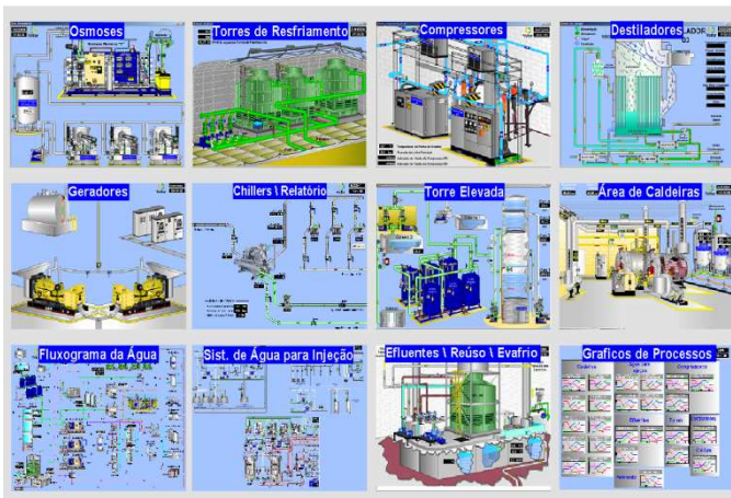
Figure 7. Utilities SCADA System to Monitor Key Process
