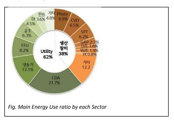
The use ratio of production equipment and utility facilities is about 4: 6. Compressor for production of compressed air (CDA) and clean room, and refrigerator for maintaining office temperature account for 33.8% of total, and SEU centered on energy saving activities have.
