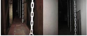
Previously the drying channel is of low energy efficiency due to too large a volume After transformation
